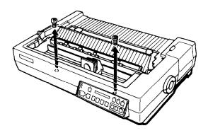
**6.** Align the pins of the paper guide cover with the slots on the printer and attach the cover. Next, attach the printer cover.
